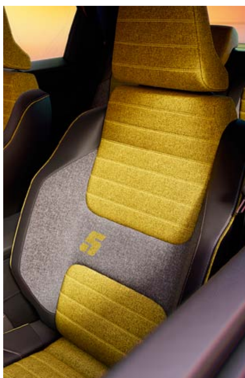
100% recycled grey and yellow marled mixed textile upholstery with yellow double topstitching / refined black bio-sourced textile
