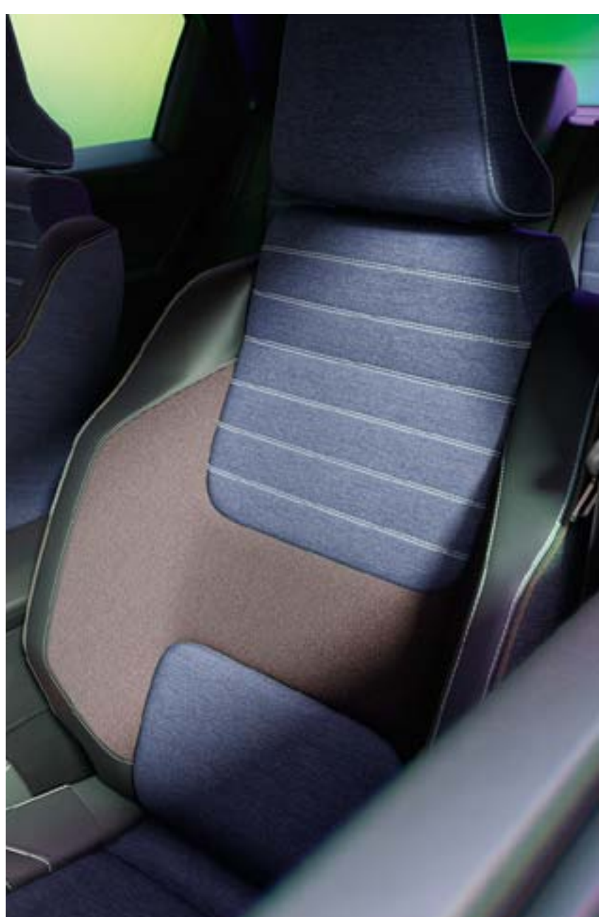
100% recycled mixed textile upholstery, denim textile with grey double topstitching / ochre central textile / black bio-sourced refined textile
